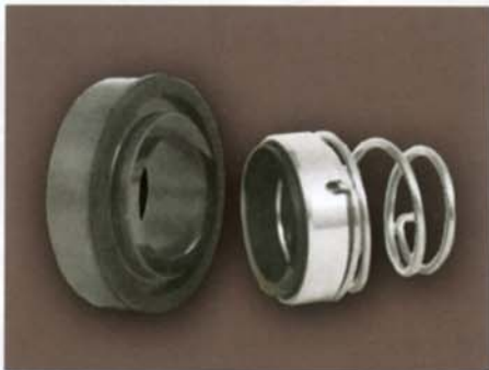
Type SW. Complete single seal for 25mm and 35mm World pumps, available with Carbon/Silicon, Silicon/Silicon or Tungsten/ Tungsten faces.
