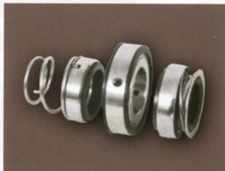
Type SWD. Complete double seal for 25mm & 35mm World pumps, available with Carbon, Silicon, Tungsten and Stainless Steel faces, dependant on the application.
