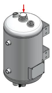
4. Fit **Ball Valve** into the small port on top of vessel marked 'FILL'
