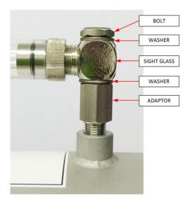
Note: Ensure the system is completely leak free before full operation. Use suitable pipe thread sealant if required.
