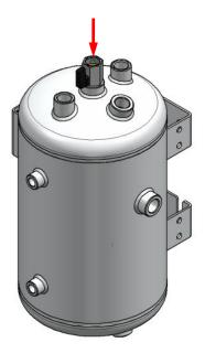
2. Fit **Seal Supply Connection** into the angled port on bottom of vessel as shown
