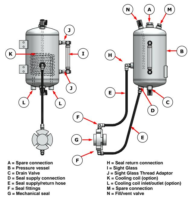
US Spec =  $\frac{1}{2}$ " fittings and connections European Spec = 12mm fittings and connections
