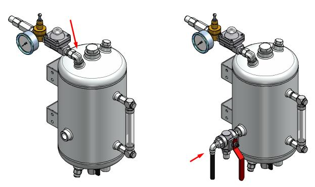
Note: Ensure the system is completely leak free before full operation. Use suitable pipe thread sealant if required.
