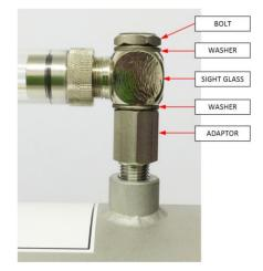
Fit 3 Way Valve Assembly into the remaining port on the side of vessel
